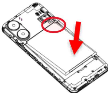
4. Put the back cover back on by pressing down on the cover's edges until the entire cover is clicked into place.
