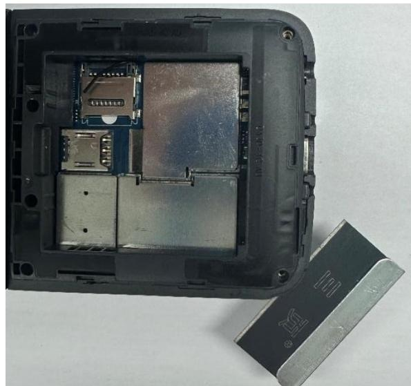
3. After the latch is fully released, carefully lift the C-shell.
