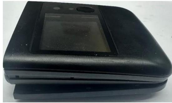
3. Starting from the bottom and working upward, gently press along the left and right edges of Shell A, allowing the clips on both sides to snap into place sequentially.
