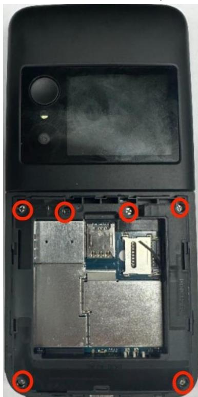
2. Insert the pry tool into the gap at the bottom of the C-shell and slowly slide it along the edge to release the clips one by one.
