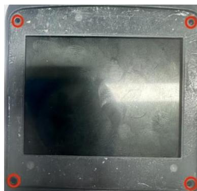
2.Align the lens precisely with the mounting groove on the B shell, ensuring the lens edge perfectly matches the shell's alignment line. Then press evenly from the center of the lens outward toward the edges.
