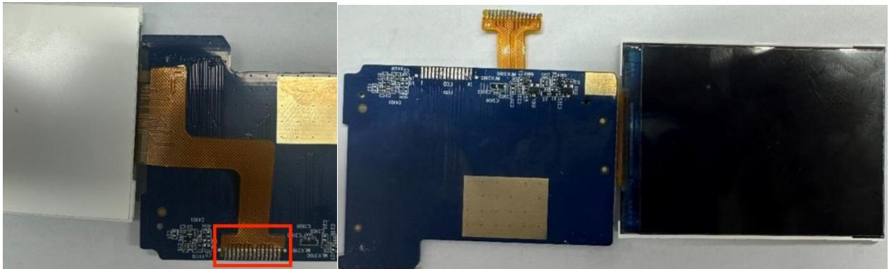
5. Apply a small amount of flux to the solder joints on the new main screen flex cable. Preheat the soldering iron to approximately 320° C. Quickly melt the solder to secure the new screen flex cable to the small board assembly. After cooling, gently press the flex cable to ensure proper contact. Inspect for any cold solder joints or bridging.
