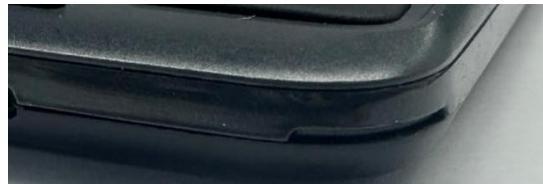
2. Insert the tip of the prying piece into the notched gap to a depth of approximately 2 mm. using the insertion point as a pivot point, slowly slide the prying piece to both sides, loosening the clips in turn.
