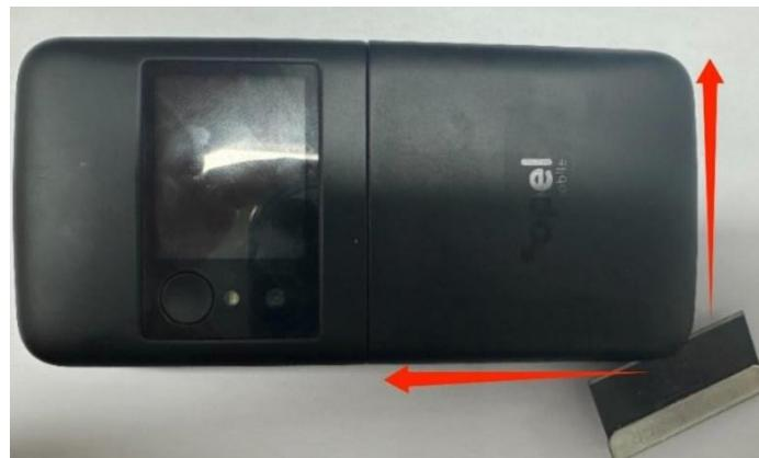
3. When the back cover is completely loose, carefully lift the battery cover.
