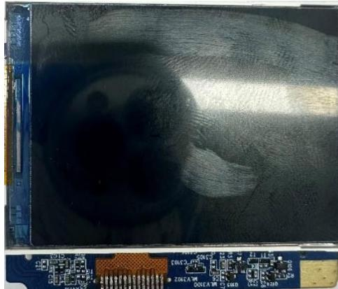
2. Align the contacts of the secondary screen FPC cable with the corresponding interfaces on the sub-board assembly. Apply flux and solder paste evenly to the surface of the solder joints on the sub-board assembly. Use a soldering iron to quickly melt the solder and complete the connection. After cooling, gently press the cable to ensure proper contact. Inspect the contacts for cold solder joints or bridging.
