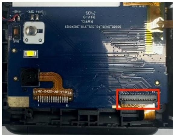
3. Insert the tip of the pry tool into the gap between the B-shell and the small board assembly. Slowly pry to release the clips. Gently flip the small board assembly along with the screen, then separate the small board assembly from the B-shell.
