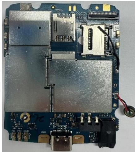
5. Locate the microphone solder joint. Preheat the soldering iron to approximately 320° C. Quickly melt the solder at the joint. Once the solder is molten, use tweezers to gently lift the connecting wire and remove the microphone.
