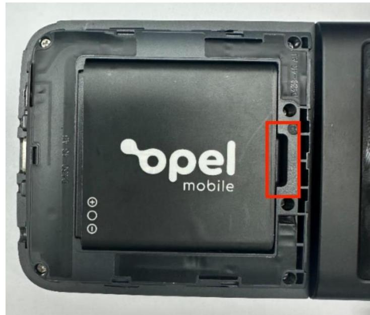
2. Insert a prying piece (or hard plastic piece) through the notch of the battery by 2-3mm. using the notch as a pivot point, gently pry the prying piece upward to separate the bottom of the battery from the body and gently remove the battery.
