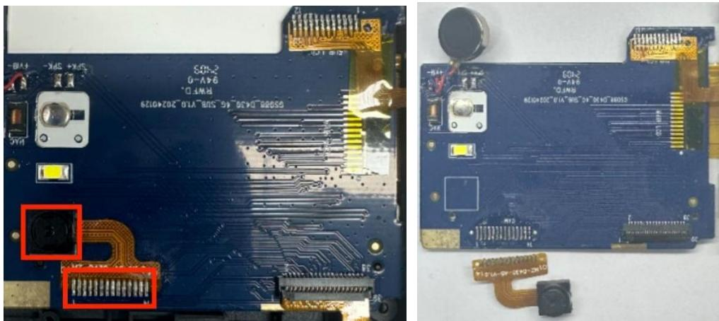
5. Locate the motor, preheat the soldering iron to approximately 320° C, quickly melt the solder at the joints, and separate the motor from the small board assembly.
