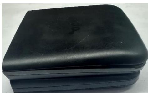
3.Press along the edges of the battery cover from left to right and from top to bottom to ensure that the edge tabs snap together one by one.
