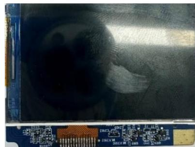
6. Apply a small amount of flux to the solder joints of the new sub-display cable. Preheat the soldering iron to approximately 320° C. Quickly melt the solder to secure the new display cable to the small board assembly. After cooling, gently press the cable to ensure proper contact. Inspect for any cold solder joints or bridging.
