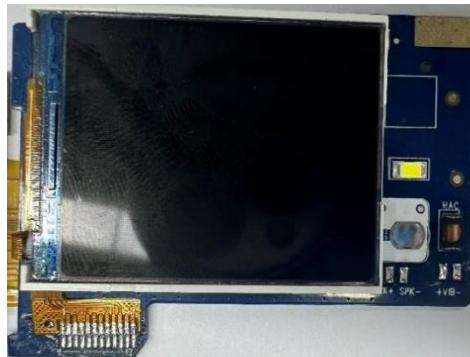
7. Insert the small board assembly into the corresponding groove in the B shell. Simultaneously insert the FPC connector into the ZF connector until the contacts are fully seated, then press the latch to secure it.
