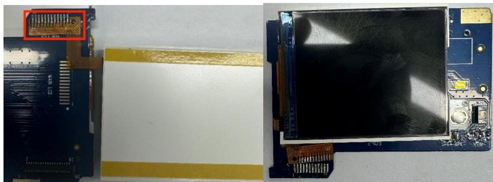
4. Apply a small amount of flux to the main display flex cable solder joints. Preheat the soldering iron to approximately 320° C. Quickly melt the solder, then gently lift the main display flex cable with tweezers to separate the old main display from the small board assembly.
