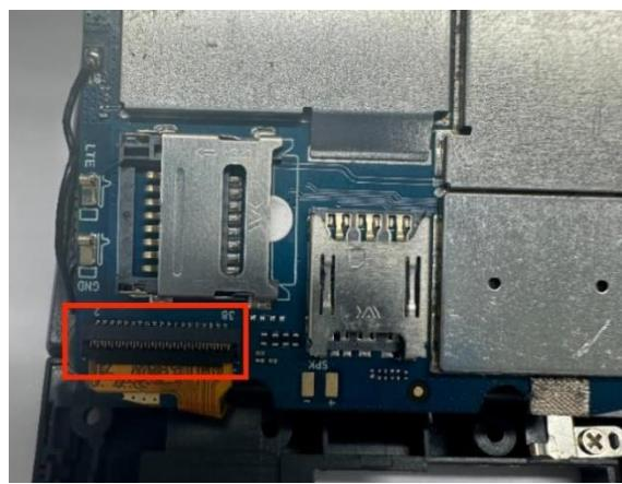
4. After confirming all clips are fully disengaged, grasp both sides of the motherboard assembly and lift it upward smoothly to remove the motherboard assembly.
