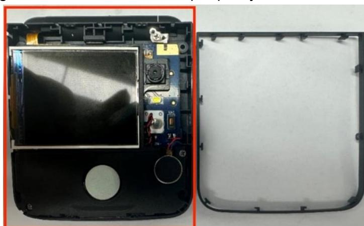
2. Pick up Shell A, align the latch at its bottom with the corresponding slot on Shell B, and insert it.
