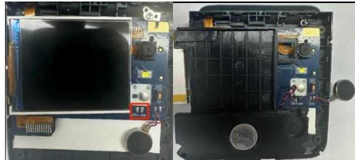
2. Align the secondary screen, motor, and camera with the grooves on the speaker module, then gently place them into position. Secure the entire module by snapping the clips into their corresponding slots.
