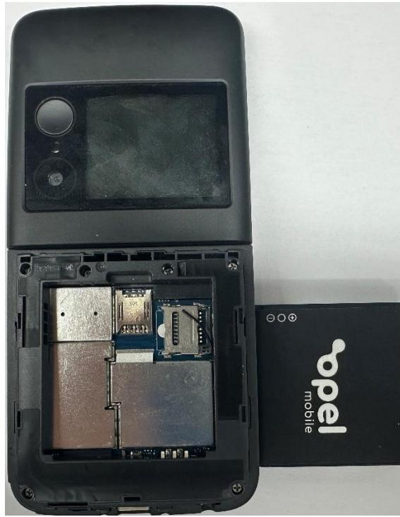
3. Take the new battery and position it with the battery contacts facing the device's battery compartment. Align the contacts on the top of the battery with the raised tabs inside the compartment. Gently push the battery into place until it is fully seated. If you encounter resistance, do not force it. Instead, check if the alignment is off.
