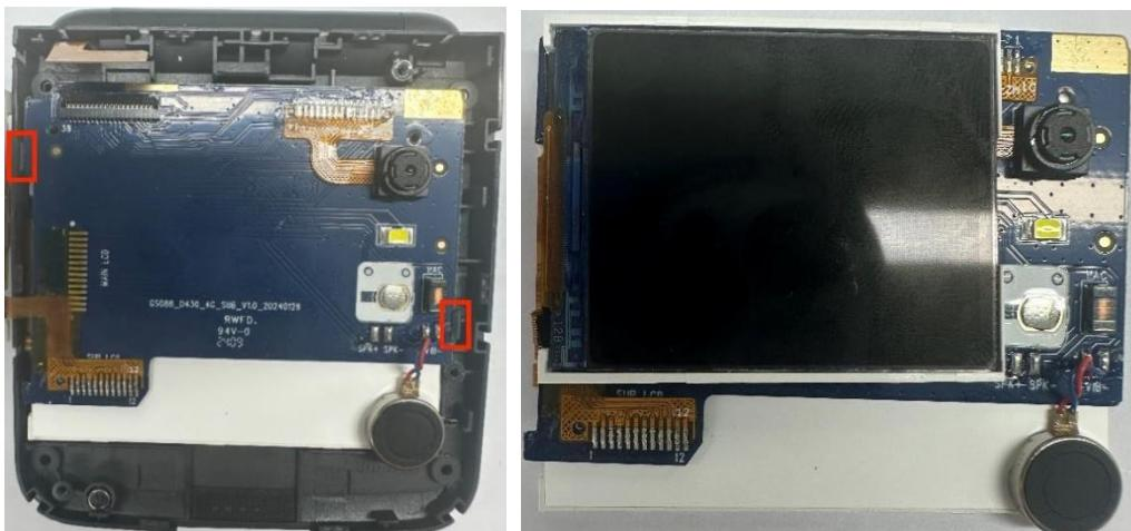
4. Locate the camera module. Using the tip of the tweezers, gently pry up one corner from the edge of the camera module and slowly remove it from the B-shell. Preheat the soldering iron to approximately 320° C. Apply a small amount of flux to the flex cable solder joints, quickly melt the solder, and separate the camera module from the small board assembly.
