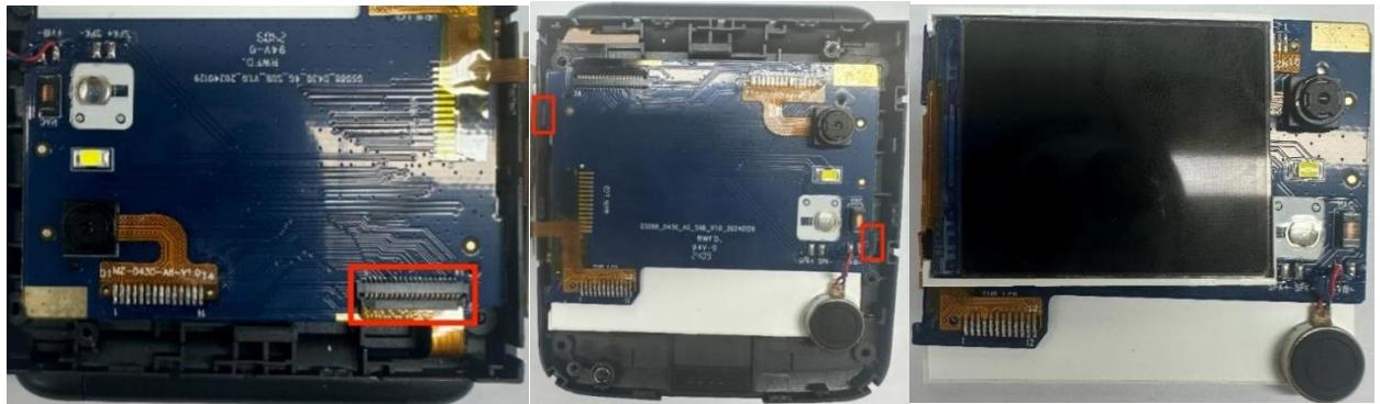
3. Apply a small amount of flux to the solder joints of the auxiliary display ribbon cable. Preheat the soldering iron to approximately 320° C. Quickly melt the solder to separate the ribbon cable from the small board assembly, then remove it from the assembly.
