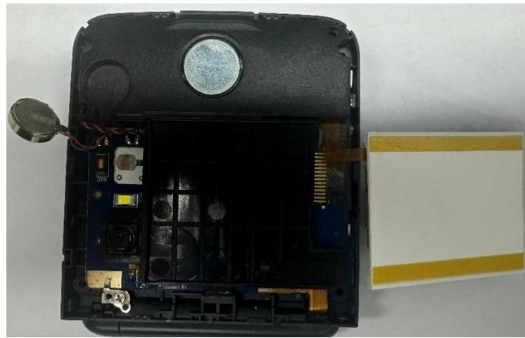
3. Flip the speaker to the left, then preheat the soldering iron to approximately 320° C. Quickly melt the solder at the speaker's joints. Once the solder is melted, gently lift the connecting wires with tweezers and remove the entire module.
