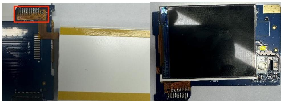
7. Locate the main display panel. Preheat the soldering iron to approximately 320° C. Apply a small amount of flux to the ribbon cable solder joints. Quickly melt the solder to separate the main display panel from the sub-board assembly.
