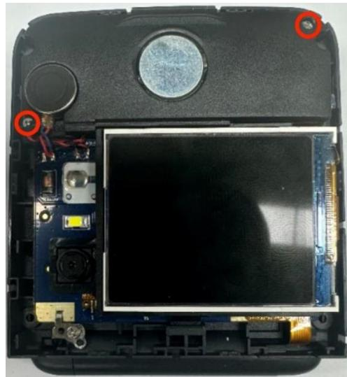
2. Flip the small screen to the right, then use tweezers to gently pry along the motor's edge. After separating the adhesive layer, remove the motor.
