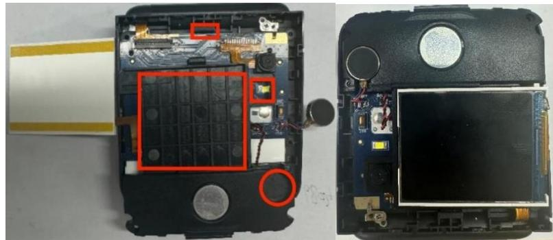
3. Screw in the screws to secure the speaker module.
