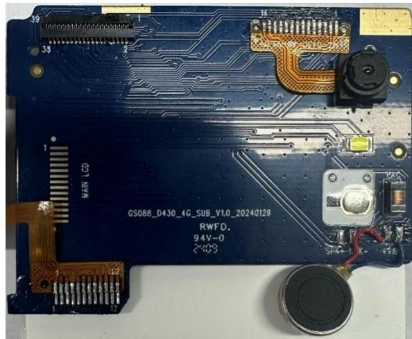
5. Insert the small board assembly into the corresponding groove in the B shell. Simultaneously insert the FPC connector into the ZF connector until the contacts are fully seated, then press the latch to secure it.
