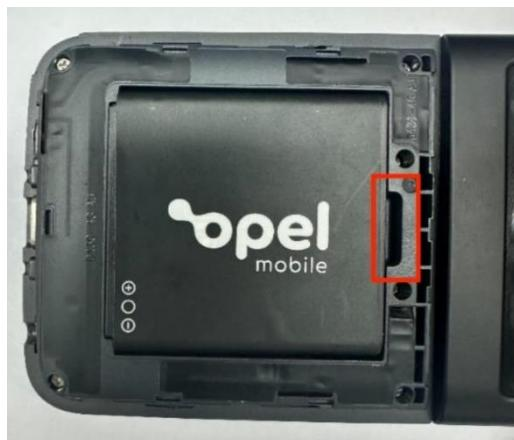
2. Insert a pry tool (or rigid plastic card) 2-3mm into the notch on the battery. Using the notch as a fulcrum, gently pry upward to separate the battery base from the device body. Carefully lift along the battery's edge to remove the old battery completely.
