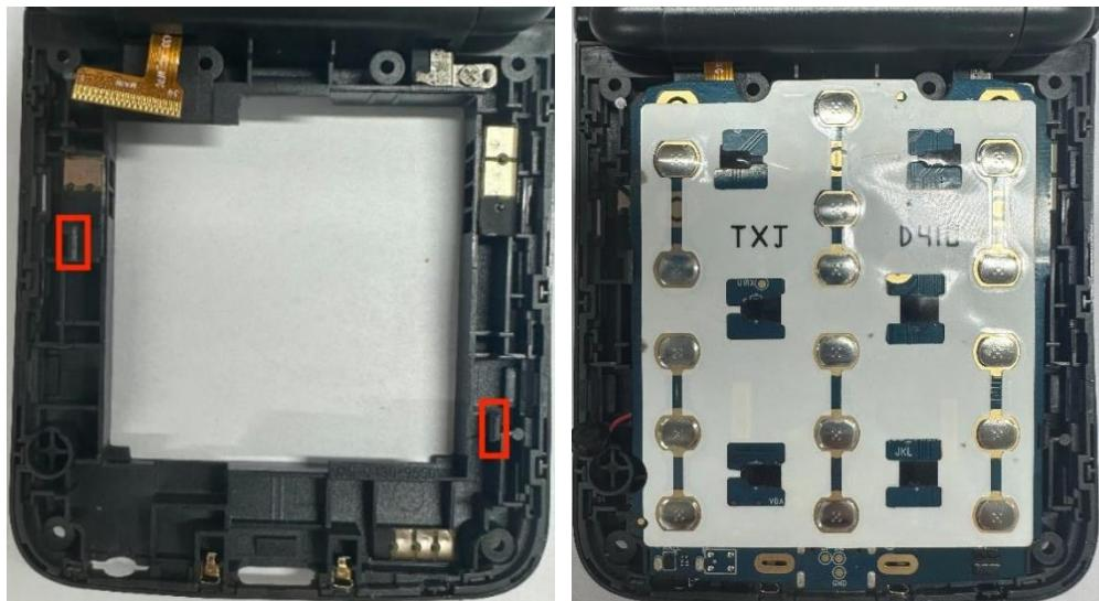
4. Using tweezers, grasp the microphone and align it with the microphone slot on the inner side of the D-shell. Slowly insert it and gently press to secure it until the microphone is fully seated in the groove.
