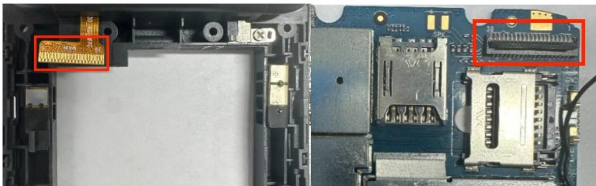
3. Align the motherboard assembly with the clips on the D-shell. Apply even pressure along the shell's edge with your fingers to snap the clips on both sides into place one after another.
