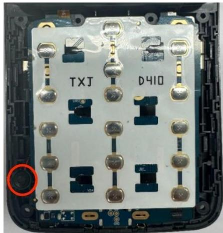
2. Insert the tip of the pry tool into the gap between the D-shell and the mainboard assembly. Slowly pry and slide along the edge to release the clips one by one.
