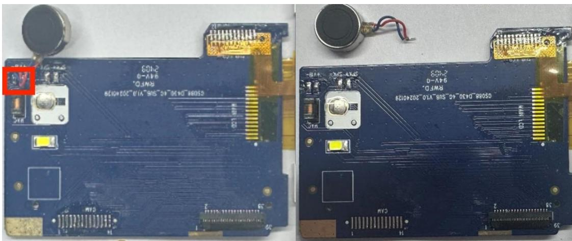
6. Locate the auxiliary display. Preheat the soldering iron to approximately 320° C. Apply a small amount of flux to the ribbon cable solder joints, quickly melt the solder, and separate the auxiliary display from the small board assembly.
